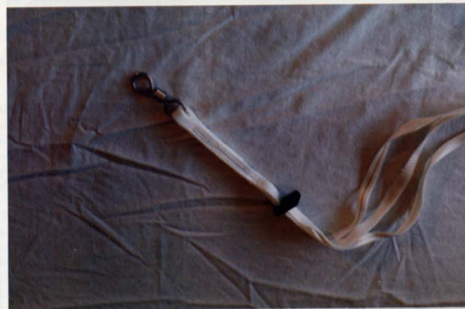
B 2 SkyAngle 60-inch 'chute. Shown are the spinner and reefing slide, the shroud line attachment at the skirt, and the shroud lines crossing at the top of the canopy.
