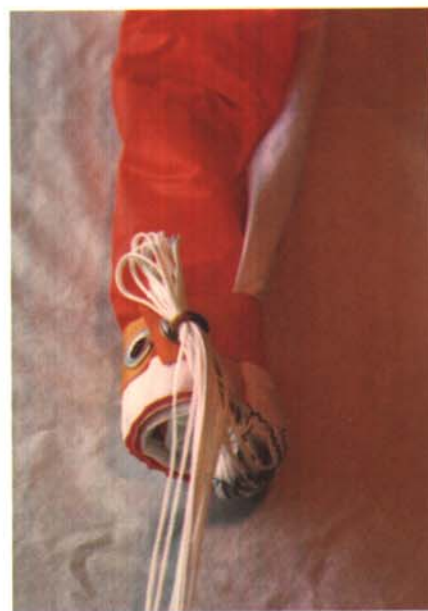
PML 84" Gradual Deployment 'chute (below) seams and shroud line attachment; shown folded with GD strap (above). This is also a very well made 'chute.
