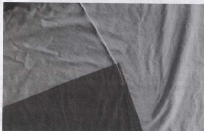
LOC/Precision 78-inch 'chute showing hem and shroud line attachment. Below: Top Flight Recovery "X" hems and shroud line attachments.
