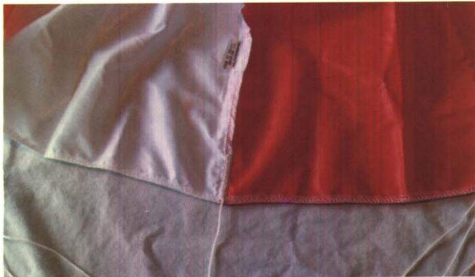
Spherachutes 36" (red and white) and 96" six-color 'chutes showing hems and shroud line attachment. These are well made 'chutes.
