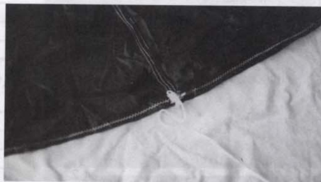
LOC/Precision 78-inch 'chute showing hem and shroud line attachment. Below: Top Flight Recovery "X" hems and shroud line attachments.
