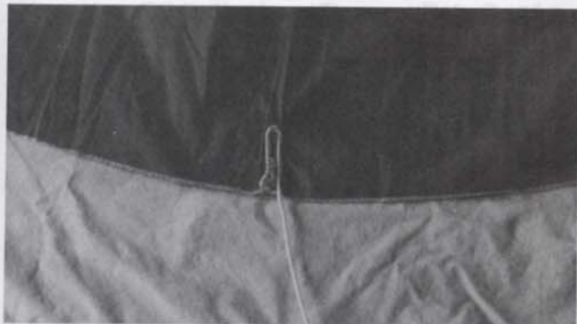
North Coast Rocketry 22" shroud line attachment. This is the weakest looking shroud line attachment of the 'chutes in the test. It showed signs of stress after the 50 MPH shock load test. Below: Rocket R&D 84-inch 'chute showing hem and shroud line attachment.
